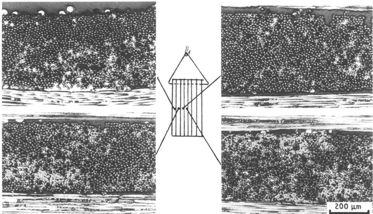
Figure 4 Effect of setting positions on infiltration (without SiC filler). 900 °C, TMS 4.5%, hold-time 1 s, 32 070 pulses.
