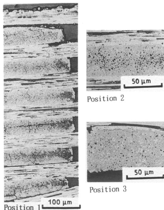
Figure 7 Cross-sectional appearance of a preform without SiC filler after 64 400 pulses of CVI at 900 °C, TMS 4.5%, hold-time 1 s.
