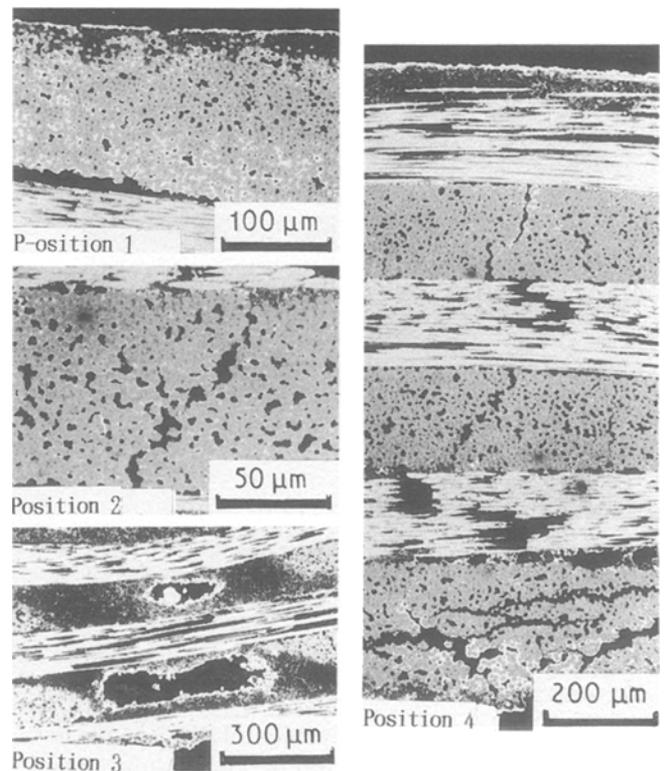
Figure 10 Cross-sectional appearance of a preform with SiC filler after  $7 \times 10^4$  pulses of CVI at 870 °C, TMS 4.5%, hold-time 0.6 s.
