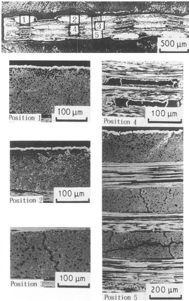
Figure 11 Cross-sectional appearance of a preform with SiC filler after  $10^5$  pulses at  $870^\circ\text{C}$ , TMS 4.5%, hold-time 0.6s.
