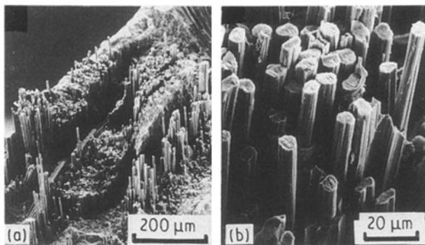
Figure 15 (a) Low and (b) high magnification views of the ruptured section. 870 °C, TMS 4.5%, hold-time 0.6 s, preform with SiC filler, after  $10^5$  pulses.
