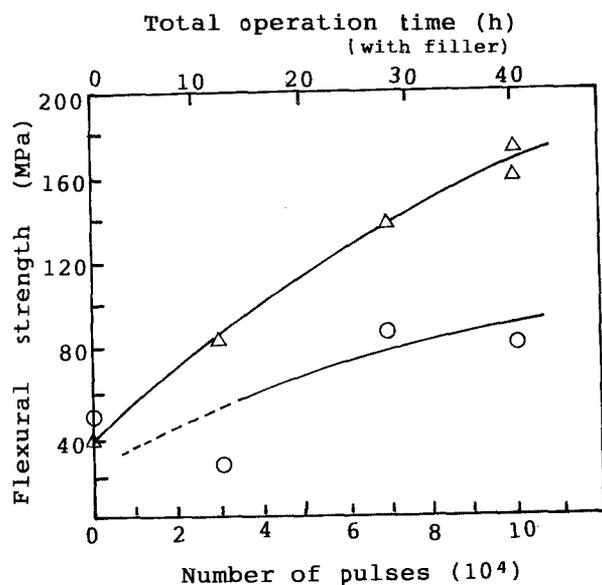
Figure 14 Relationship between flexural strength and number of pulses (○) without filler, (△) with filler.
