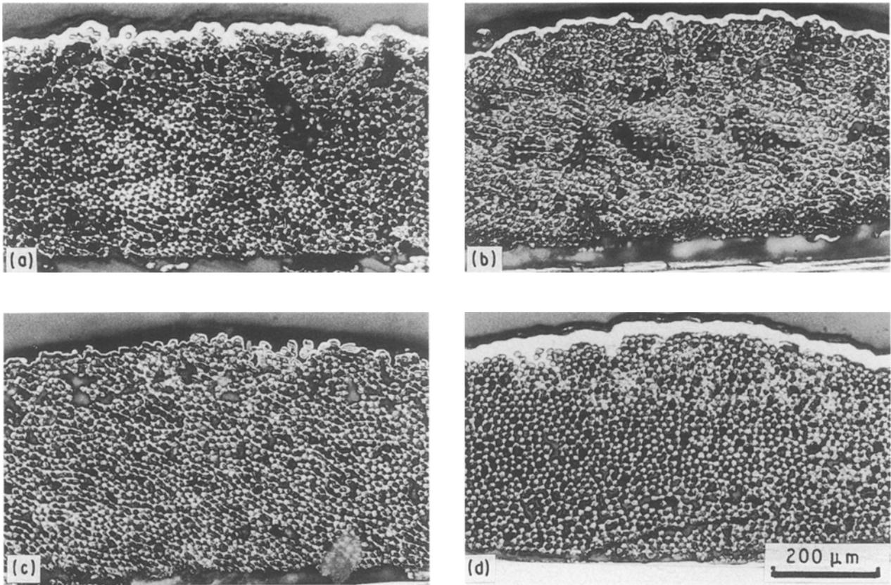
Figure 3 Dependence of infiltration on the deposition temperature and number of pulses. (a) 1300 °C, TMS 7%, hold-time 0.7 s, 1000 pulses, (b) 1200 °C, TMS 7%, hold-time 3.5 s, 1200 pulses, (c) 1100 °C, TMS 7%, hold-time 2.5 s, 1200 pulses, (d) 1000 °C, TMS 4.5%, hold-time 2.5 s, 8500 pulses.
