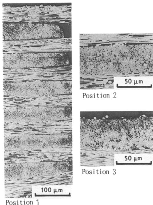
Figure 6 Cross-sectional appearance of a preform without SiC filler after 32 070 pulses of CVI at 900 °C, TMS 4.5%, hold-time 1 s.
