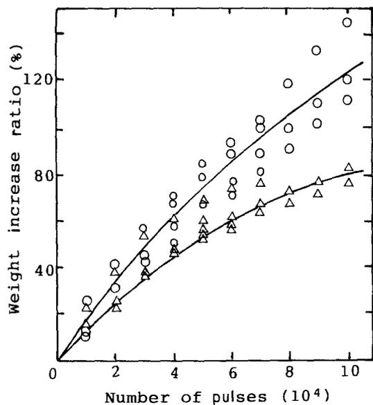
Figure 5 Relationship between weight increase and number of pulses (○) without SiC filler, 900 °C, TMS 4.5%, hold-time 1 s, (△) with SiC filler, 870 °C, TMS 4.5%, hold-time 0.6 s.
