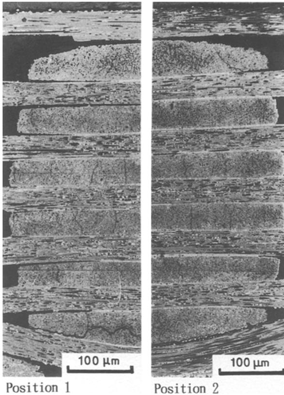
Figure 8 Cross-sectional appearance of a preform without SiC filler after 99 800 pulses of CVI at 900 °C, TMS 4.5%, hold-time 1 s.
