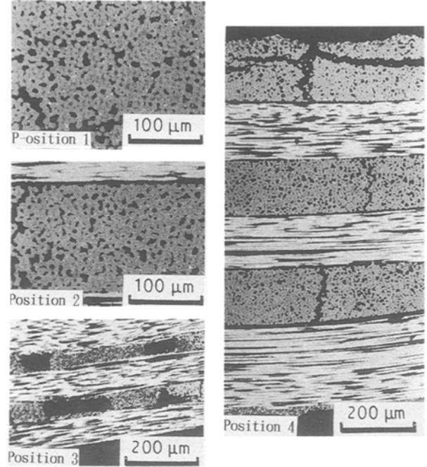
Figure 9 Cross-sectional appearance of a preform with SiC filler after  $3 \times 10^4$  pulses of CVI at 870 °C, TMS 4.5%, hold-time 0.6 s.
