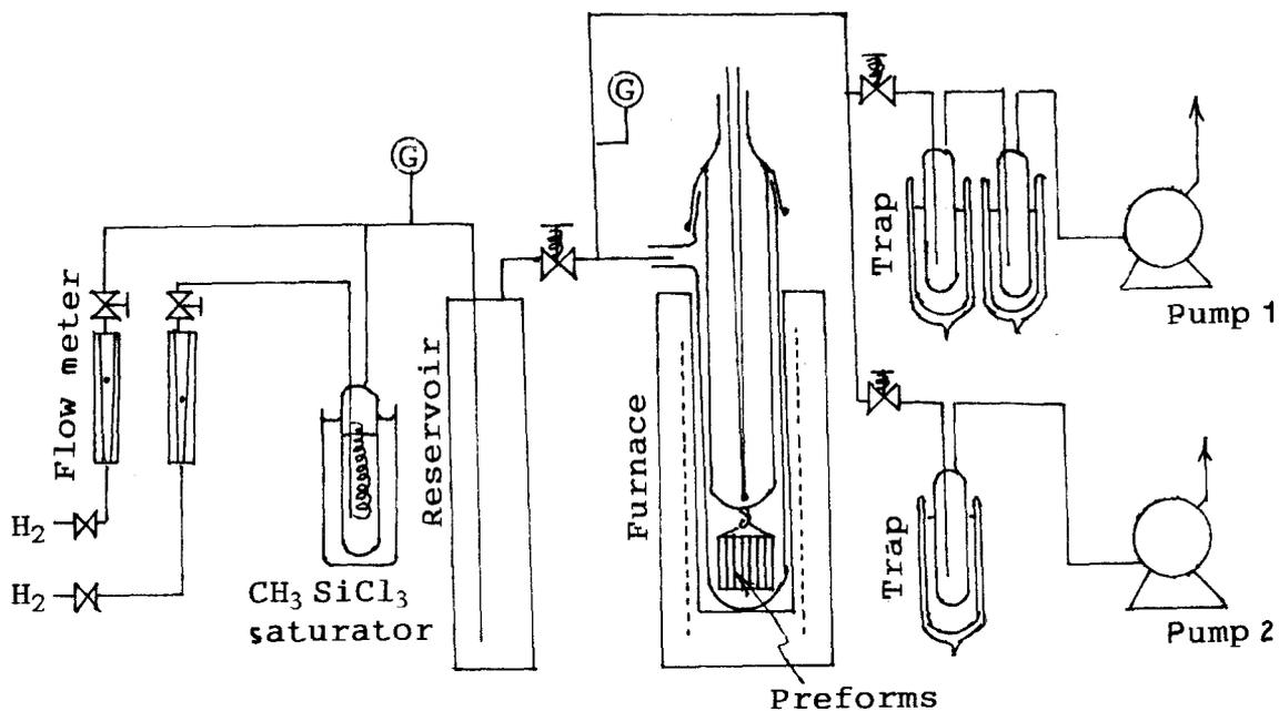
Figure 1 Apparatus for pulsed CVD of SiC to 3D-C/C preforms.
