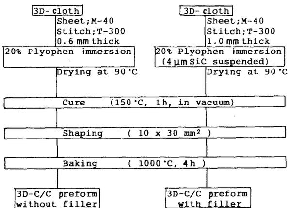
Figure 2 Preparation steps of preforms.
