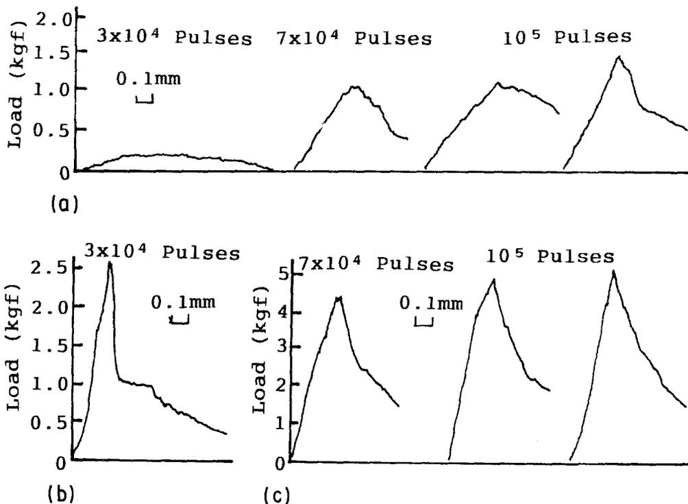
Figure 13 Stress-strain curves during the three-point flexural strength testing, (a) without filler,  $10 \times 30 \times 0.6 \text{ mm}^3$ , (b, c) with filler,  $10 \times 30 \times 1.0 \text{ mm}^3$ .
